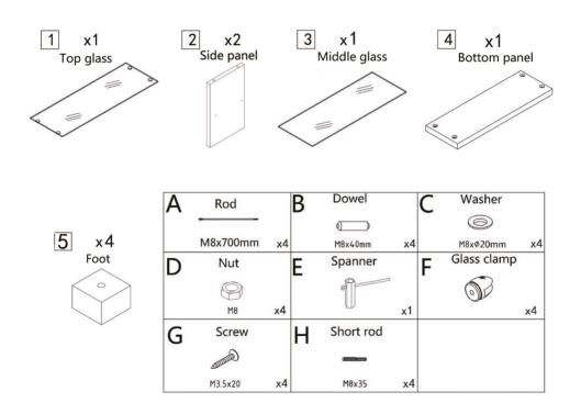
**NOTE:** The quantities above are the correct amount to complete the assembly. In some cases more fittings may be supplied than are required.
