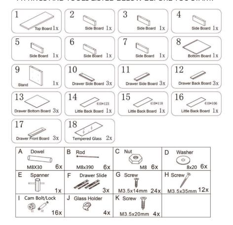
**NOTE:** The quantities above are the correct amount to complete the assembly. In some cases more fittings may be supplied than are required.
