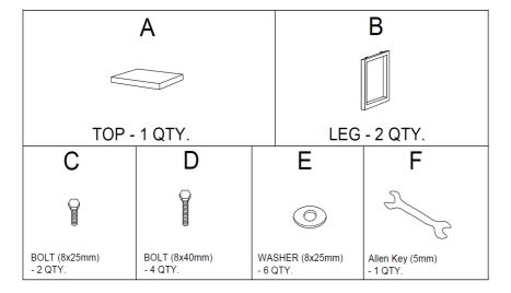
**NOTE:** The quantities above are the correct amount to complete the assembly. In some cases more fittings may be supplied than are required.
