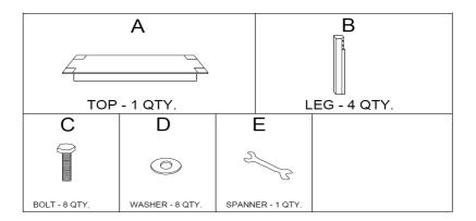
**NOTE:** The quantities above are the correct amount to complete the assembly. In some cases more fittings may be supplied than are required.
