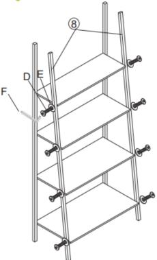
Attach 2x front legs [8] to the shelves using 1 x washer [E] followed by 1 x bolt [D] on each side of each shelf - 8 in total. Tighten with Allen key [F].
